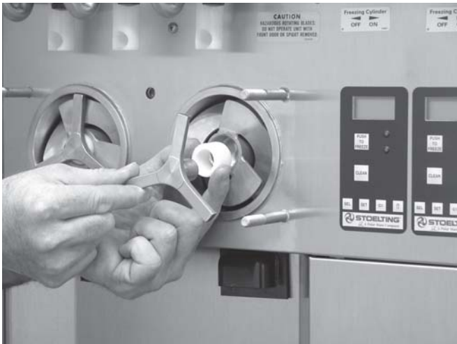
Figure 20. Removing Auger Supports
