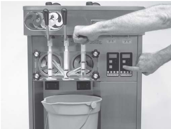
Figure 13. Spigot Opened and Solution Draining
