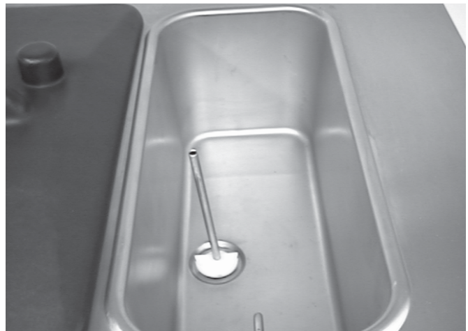
Figure 24. Install Mix Inlet Regulators
